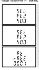
Use the MDA and PY buttons to select the menu option. The screen will show the current setting. The default value is 400V.
