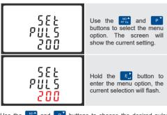
Use the and p buttons to choose the desired pulse rate. To save the new setting, hold the b button for 3 seconds until the selection stops flashing.
