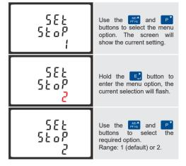
On completion of the entry procedure, hold the E button for 3 seconds until the selection stops flashing
