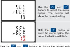
Use the and buttons to choose the desired pulse rate. To save the new setting, hold the button for 3 seconds until the selection stops flashing
