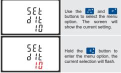
Hold the MA button for 3 seconds to exit the set up menu
