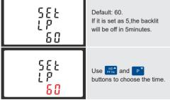
Press to confirm the setting and press MA to return to the main set-up menu.
