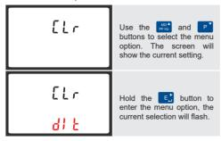
Hold the button to confirm the setting and press WA to main set up menu.
