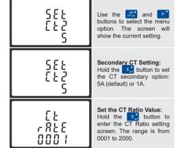
The CT Rate is the CT Primary divided by the CT Secondary. For Example: 200/5A Current Transformers - 200÷5=40, so the CT Rate would be 0040 and the CT2 would be 5. On the MID Version, you can only program the CT Rate ONCE.
