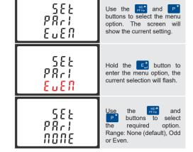
On completion of the entry procedure, hold the button for 3 seconds until the selection stops flashing
